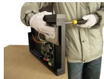
③fix the screw of hard disk
