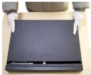
②disassemble the cover
