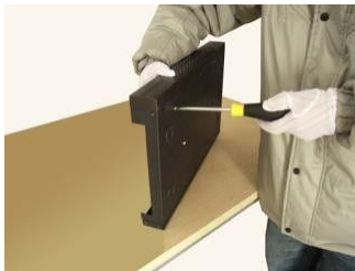
④fix the screw of hard disk
