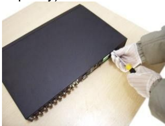
①disassemble the screw
