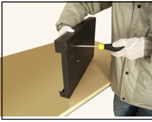
④fix the screw of hard disk
