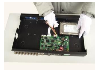
⑥connect the power wire
