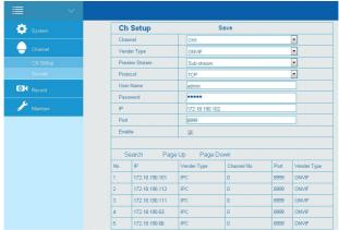
In this section, we can set the parameters of IPC protocol type, preview stream, access protocol, user name, password, IP address, port and so on.
