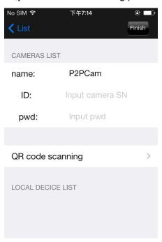
Edit the camera name,input the username,pwd,you can input the camera SN manually or scan the QR code directly,as is shown in the following picture:
