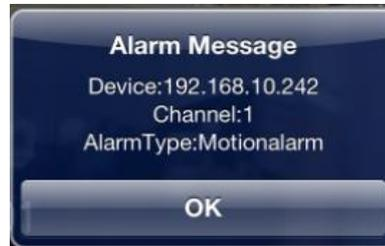
This is an example of Motion detection alarm; you can set the sensitivity in the DVR
