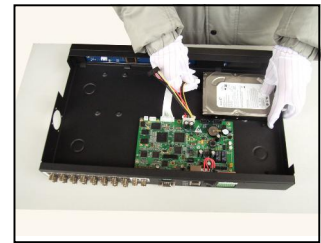
⑥connect the power wire
